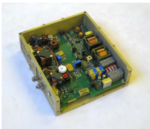
The electrical model of the Low Voltage DC/DC converters including the variable gate voltage of the mass spectrometer
