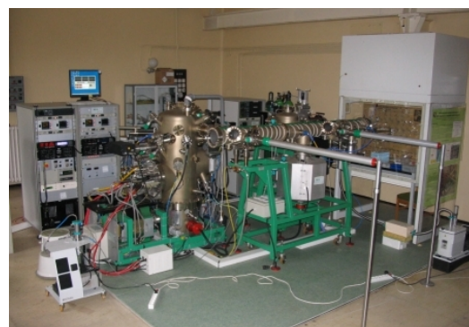
The MECA-2000 molecular beam epitaxy facility for preparing metallic thin-film samples under ultrahigh-vacuum conditions
