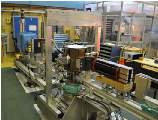
The GINA reflectometer with newly installed electromagnet and closed cycle He-cryostat at the Budapest Neutron Centre (BNC).
