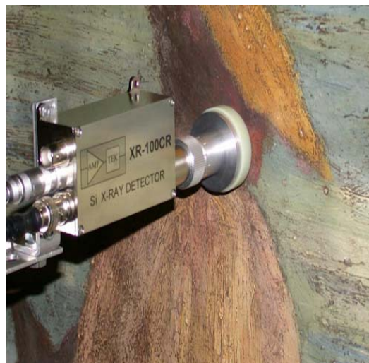
The XR100CR Si X-ray detector fitted with a ^{109}\text{Cd} source doing XRF on a painting. This picture appears by permission on the home page of Amptek® ( http://www.amptek.com/art.html ).
