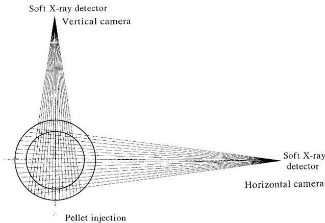
FIG. 1. Experimental setup. Both the horizontal and the vertical camera had 16 viewing chords each.
