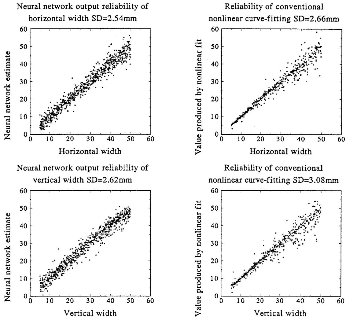
FIG. 4. Performance of the neural networks and conventional curve fitting on width parameters. On each of the figures the network output or the results of the curve fitting are plotted on the vertical axis against the generating parameters of the samples (desired output). Standard deviation from the desired output is written on top.
