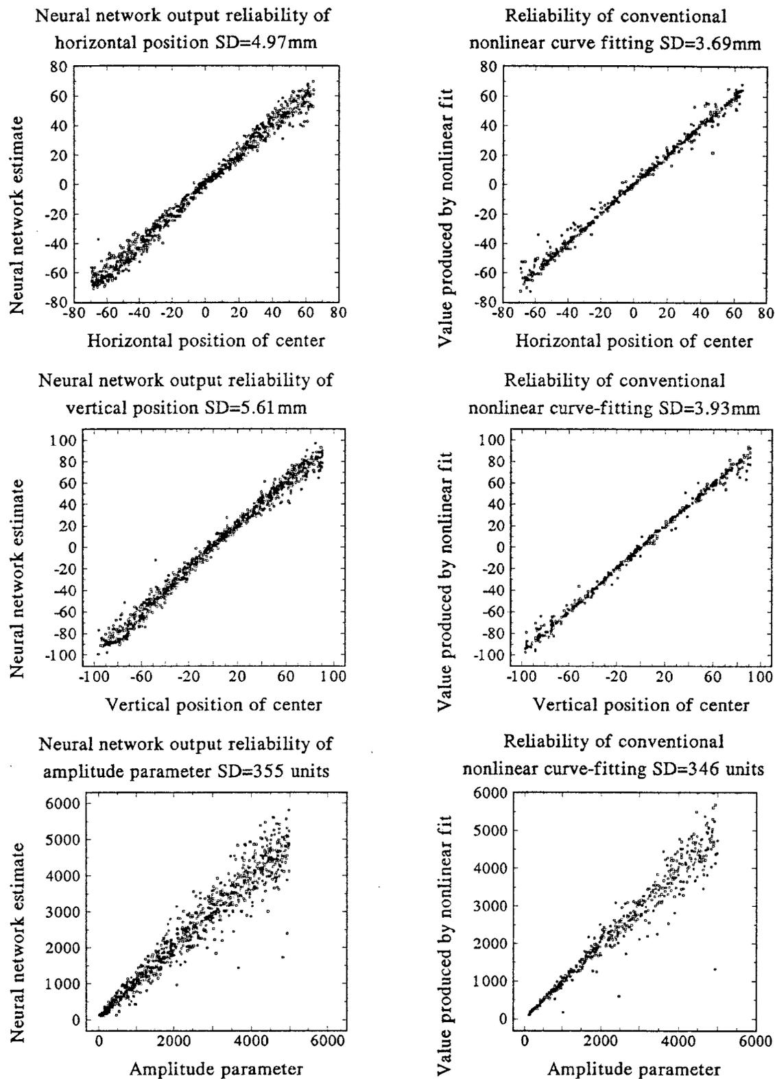
FIG. 3. Performance of the neural networks and conventional curve fitting on position and amplitude parameters. On each of the figures the network output or the results of the curve fitting are plotted on the vertical axis against the generating parameters of the samples (desired output). Standard deviation from the desired output is written on top. Note that the plots of the conventional fit contain only half the number of points as the neural network plots.
