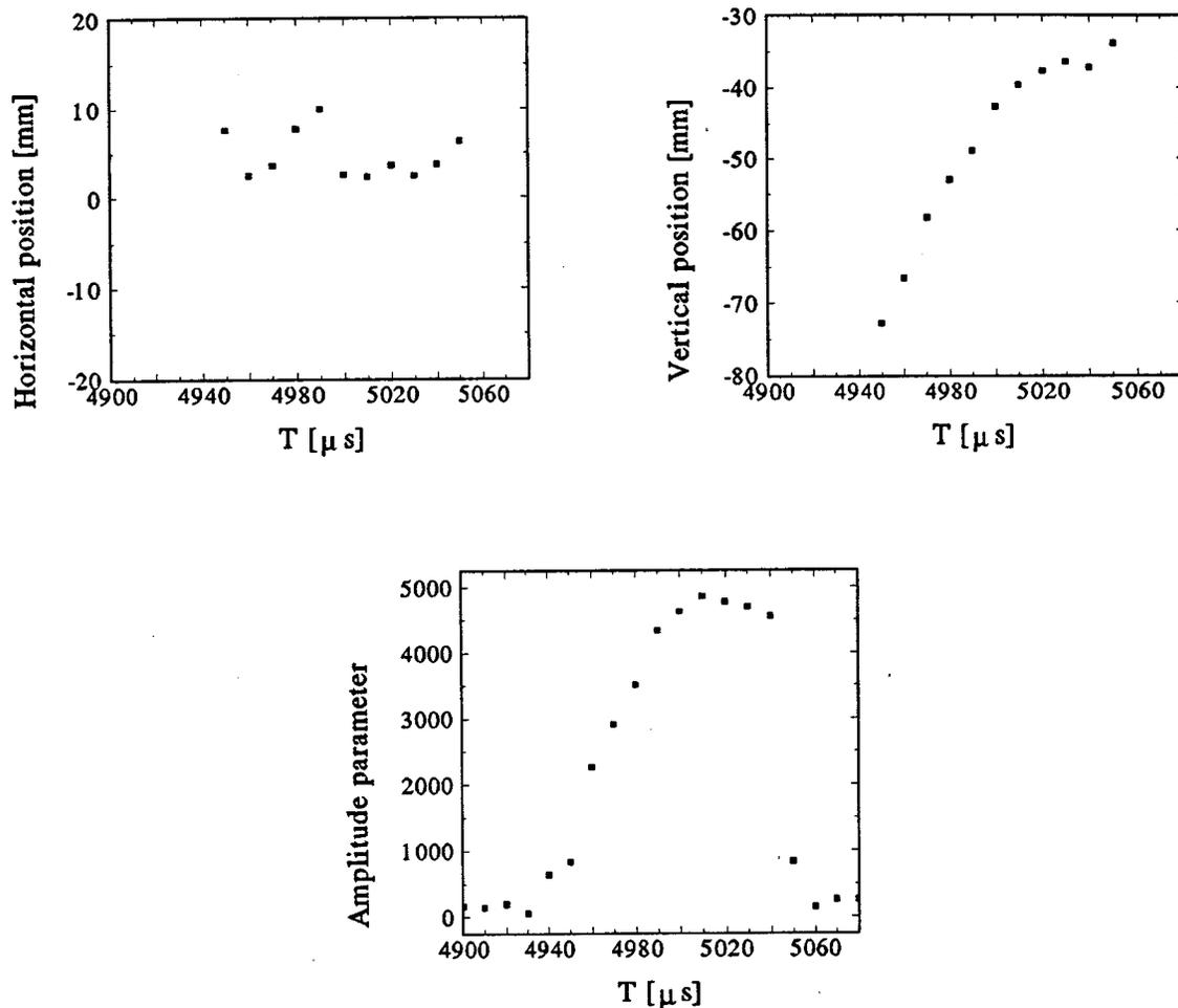
FIG. 5. Results of tomographic data processed by neural networks. The position parameters can be seen to correspond to a localized distribution moving into the plasma from below in the vertical direction, while the amplitude parameters correspond to a sudden increase in radiation from impurity ions.
