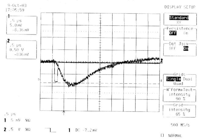
• Rise-time of 500ns was bit too long for triggering in NA49. Would need to replace shaper/amplifier of the modules to make it more suitable.
