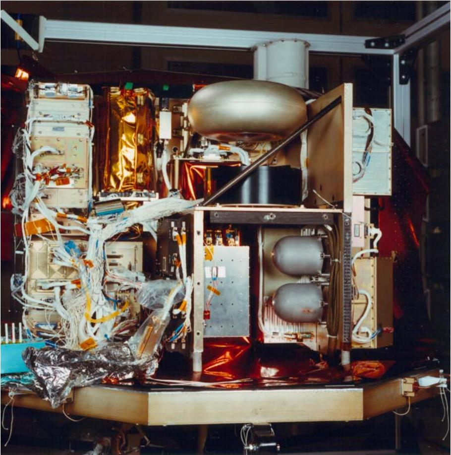
Figure 5. Internal compartment of the Lander Electrical Qualification Model (EQM), during integration.
