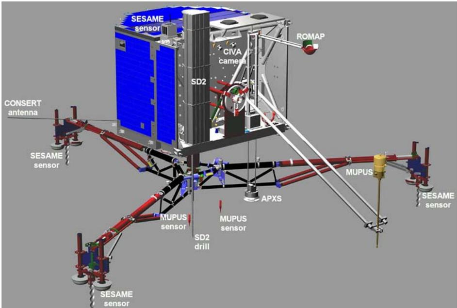
Figure 3. Schematic view of the Philae spacecraft. The figure shows the overall structure, the subsystems and the experiment compartment of the Lander. The location of some scientific instruments and their sensors are indicated; some are not visible in the drawing: specifically, the instruments in charge of analyzing the samples distributed by the SD2 (CIVA, COSAC, PTOLEMY), and the down-looking camera (ROLIS).
