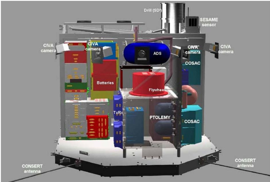
Figure 4. Side view schematics of the inner structure of the lander compartment showing the location of COSAC and PTOLEMY systems, the CONSERT antennas, the SESAME dust sensor and various CIVA cameras.
