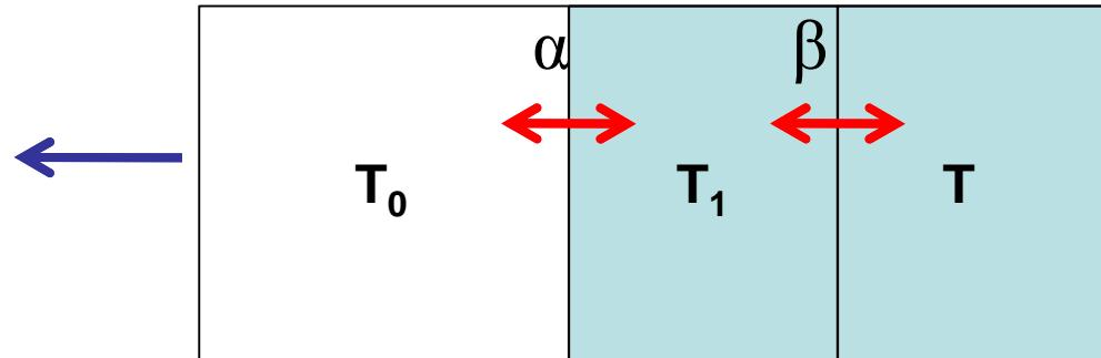
$$\frac{1}{\alpha + \beta} \ddot{T} + \dot{T} = -\frac{\alpha\beta}{\alpha + \beta} (T - T_0)$$
