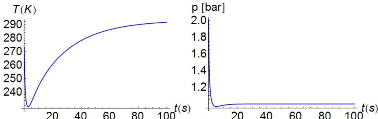
Fast mechanical equilibration: adiabatic process followed by an isobaric one: no oscillations
