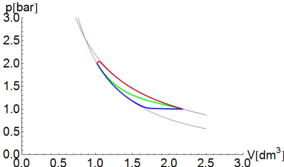
The isothermal (red), adiabatic-isobaric blue and mixed (green) processes together with the  $T = T_a$  isotherm and  $p = p_i(V/V_i)^\kappa$  adiabatic curves (thin lines) on the p-V plane.
