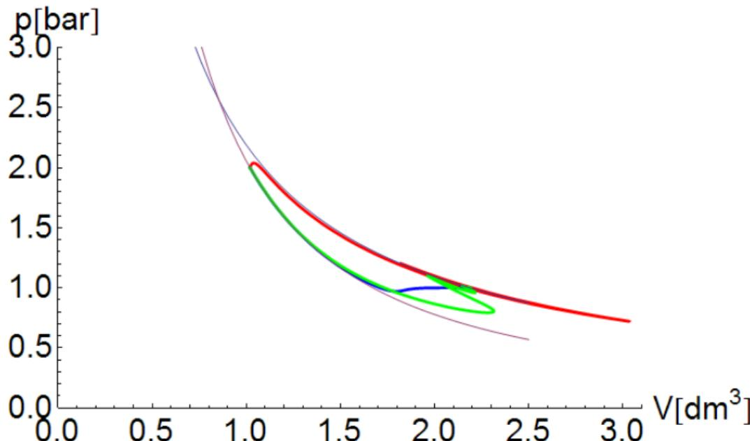
The isothermal (red), adiabatic-isobaric blue and mixed (green) processes together with the  $T = T_a$  isotherm and  $p = p_i(V/V_i)^\kappa$  adiabatic curves (thin lines) on the p-V plane. Oscillations galore.
