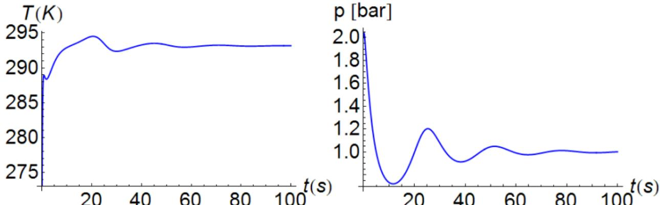
Fast thermal and slow mechanical equilibration : isothermal oscillations
